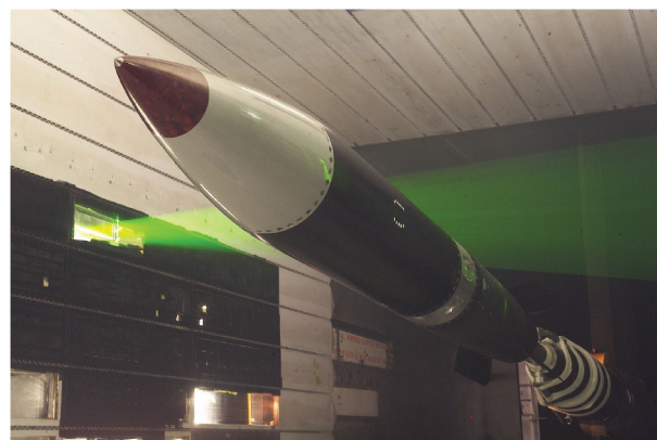
Fig. 5 Photograph of the laser sheet position relative to the wind-tunnel model.
